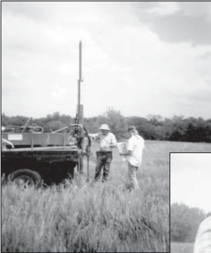
(Left) A Natural Resources Conservation Service (NRCS) Giddings rig was used to ground truth a number of the anomalies detected during the geophysical survey.
